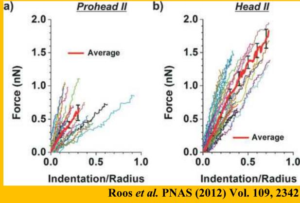
The AFM nanoindentation experiments on bacteriophage HK97 show a surprisingly complex maturation pathway in which the fragile Prohead II (P-II) is being strengthened by: i) an increase in Young's modulus, ii) an increase in ultimate strength and iii) astance against material fatigue. The resulting particle is called Head II (H-II).
